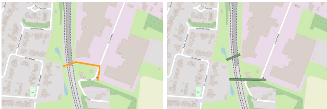
Figure 24: In orange, the location of the real culvert. In green, the simulated culvert.
