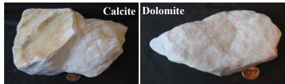
Figure 3.2. Rock samples of moura calcite marble and chemical pure dolomite before crushed.
