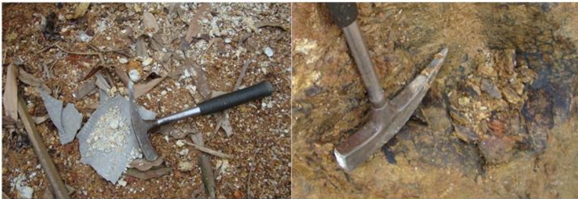
Figure 0.8: Small block size that has large Intact Rock Strength (IRS) from geotechnical unit(s) of Cut slope Y1
