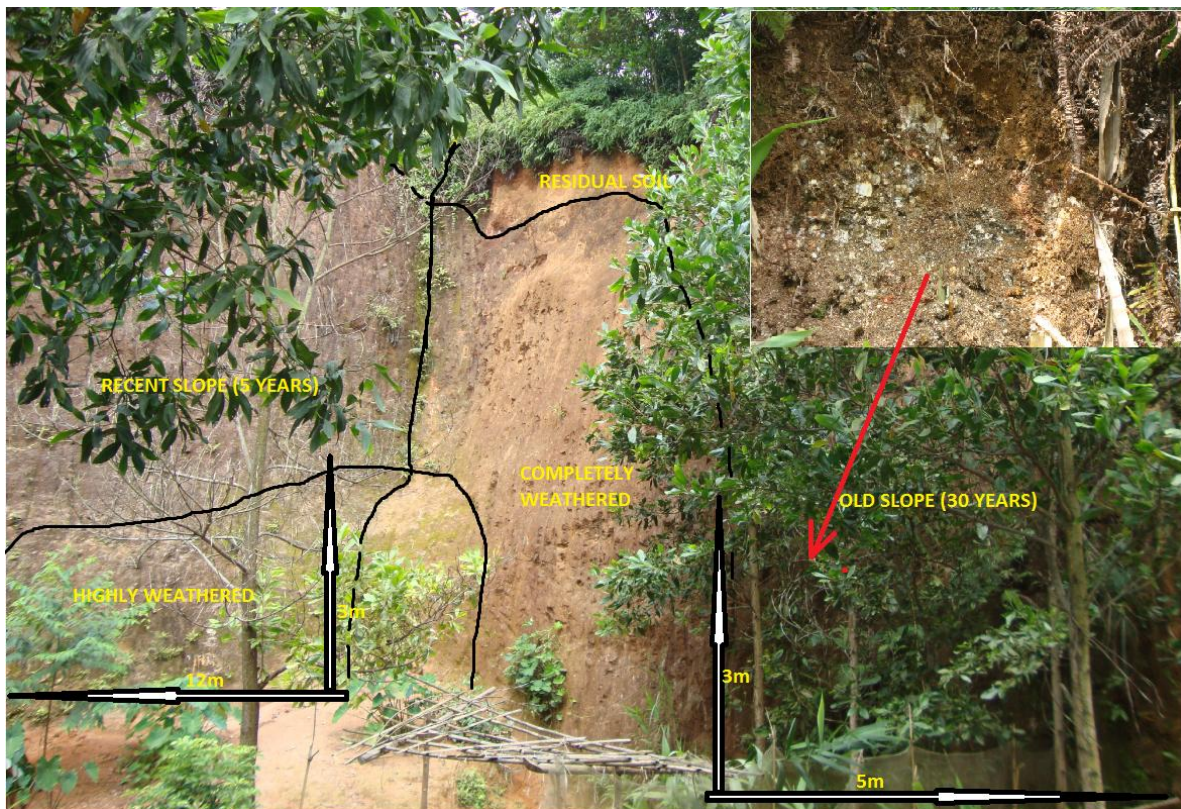
Figure 0.19: The different lithologies and degrees of weathering of Slope Y11 (Direction of view - 330^{\circ} )
