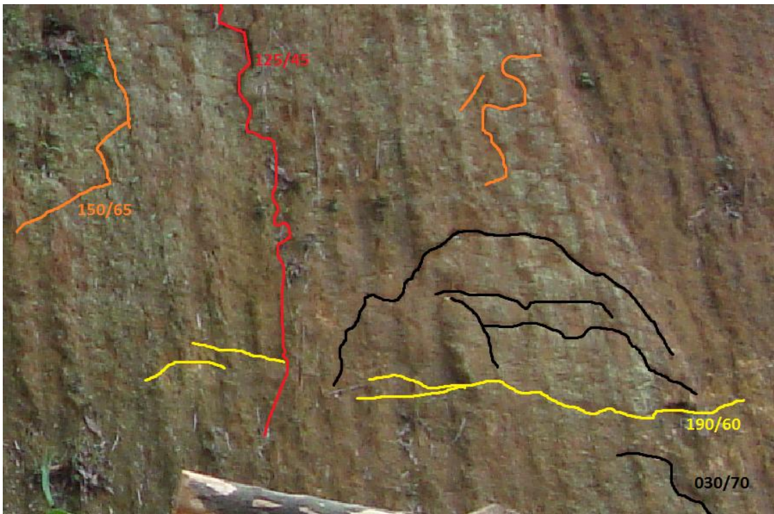
Figure 0.31: Discontinuities' orientation for the geotechnical units of Slope Y28
