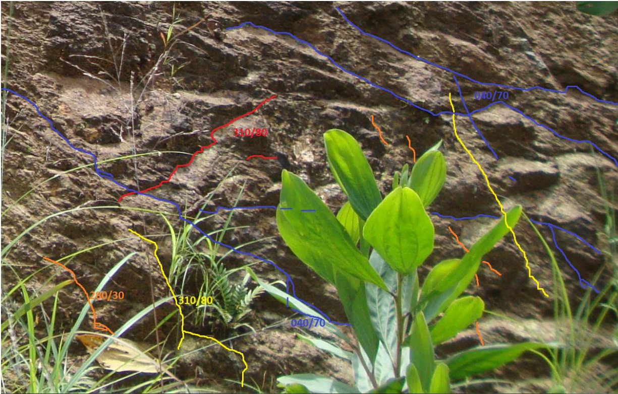
Figure 0.15: Discontinuities' orientation for the geotechnical units of medium part of Slope Y4
