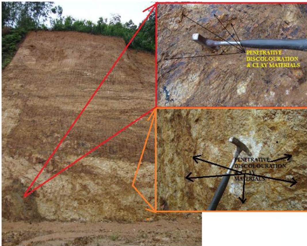
Figure 0.55: Typical moderately weathered rock materials from the research area - cut slope Y1 - 27/09/2010 - 10.00hrs; Scale - 1:6000)
