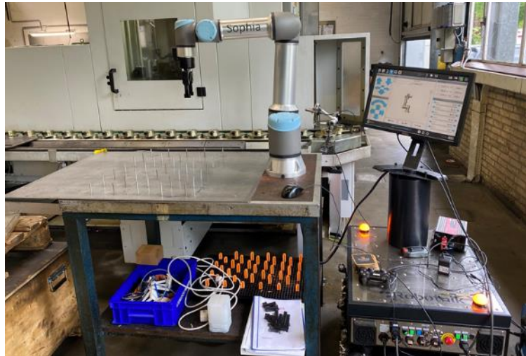
Figure 19: Cobot Sophia with dedicated table to store workpieces
