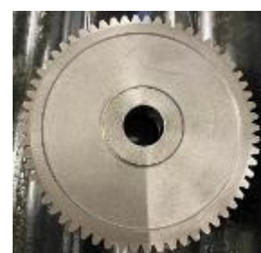
Figure 9: Gear after heat treatment
