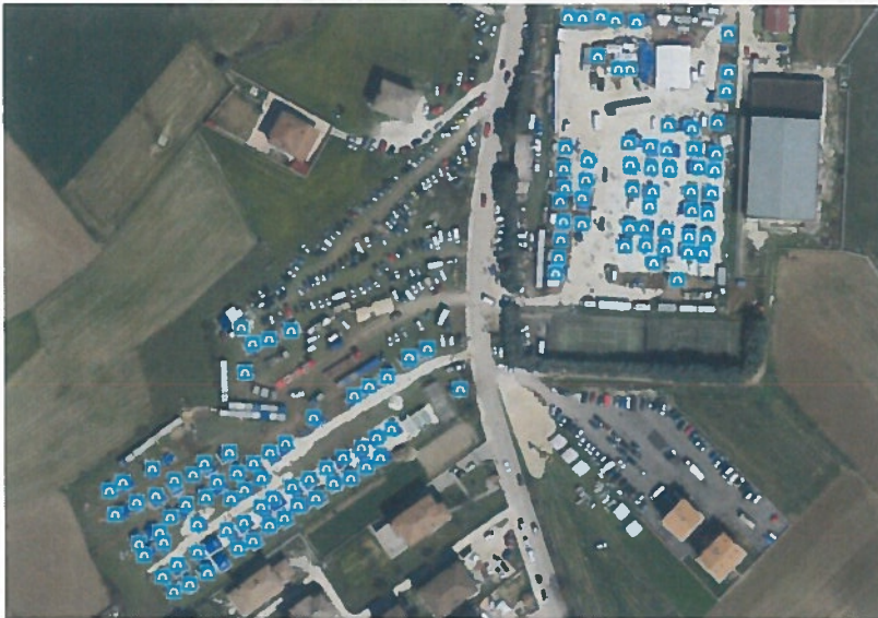
Figure 3-5: Tent WMS layer and 8 April aerial photo
