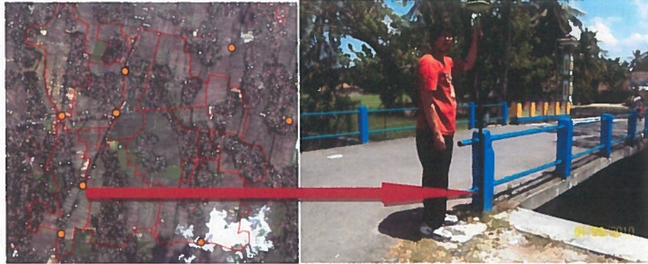
Figure 4-2: The georeference of quickbird imagery, and the measure of position in the field.
