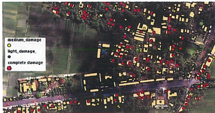
Figure 4-3: Sample of building footprint digitations in scenario before earthquake at Karasan sub village
