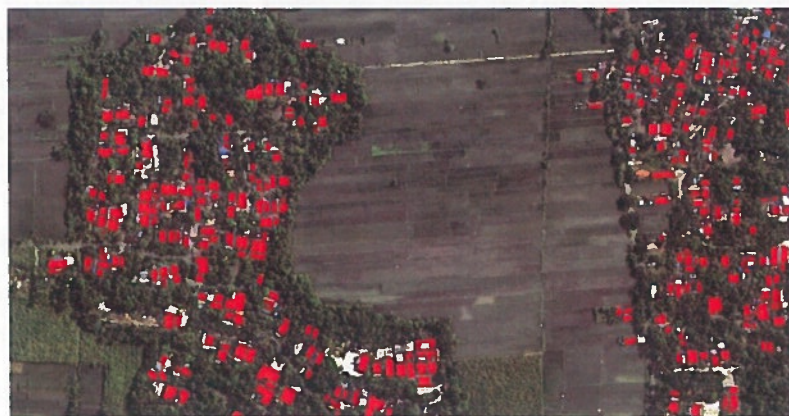
Figure 4-4: Sample of digitations building footprint after earthquake in Bolon subvillage
