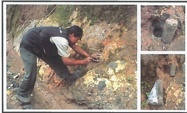
Figure 3.3. Rock mass sampling using iron pipe blown by geological hammer at saprolith portion of regolith.
