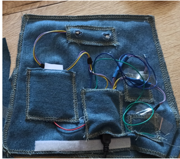
FIGURE 9.2: Overview of lower layer with components pouches
