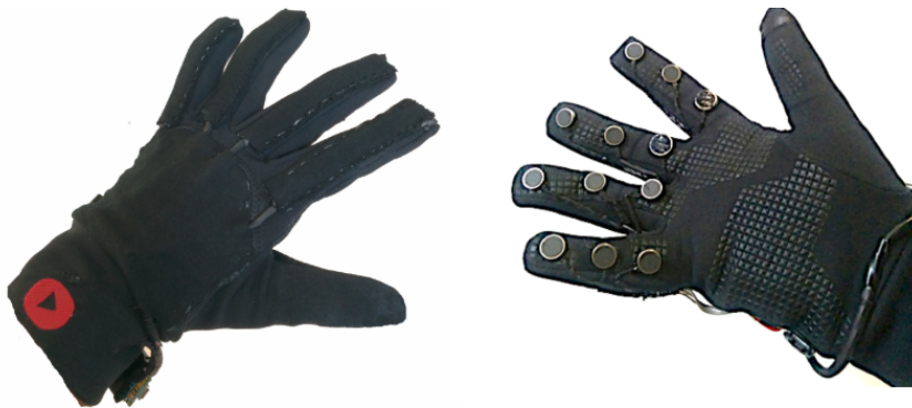
(B) Prototype Flex-n-Feel, left is the glove administrating a touch and on the right is the glove receiving the touch. [41]
