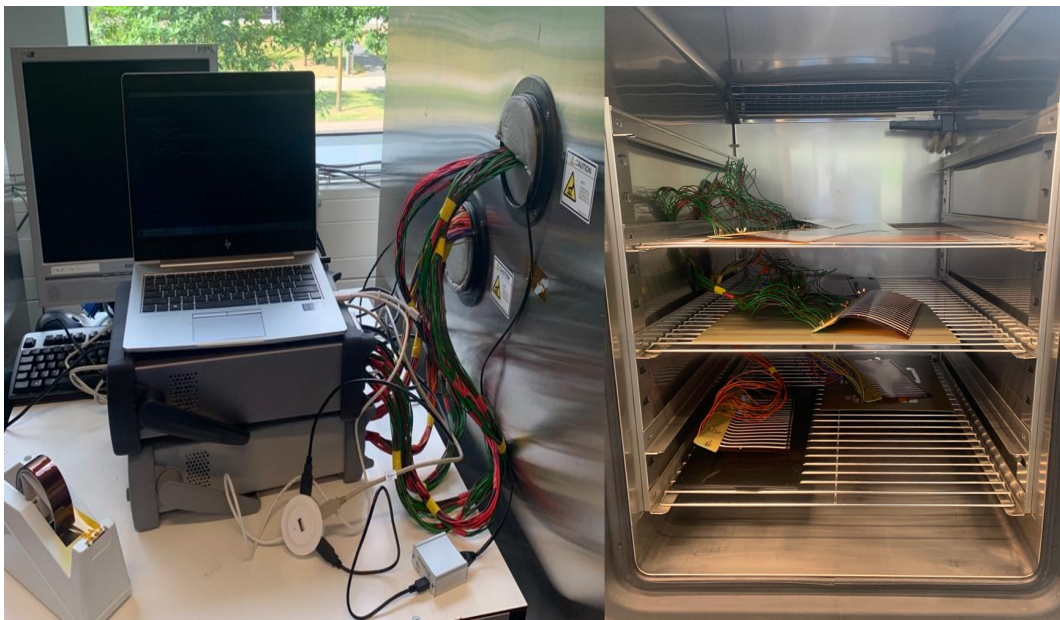
Figure 2.5: Climatic chamber setup for high humidity test.
