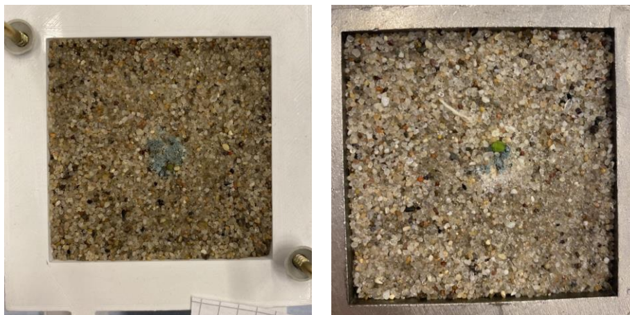
Figure 16 Samples showing mold growth around the seed.
