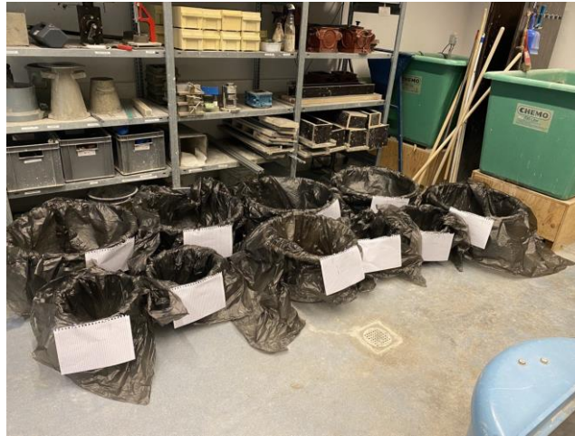
Figure 6 Buckets containing sand divided by particle size ranging from 1.5 mm to 0.125 mm.
