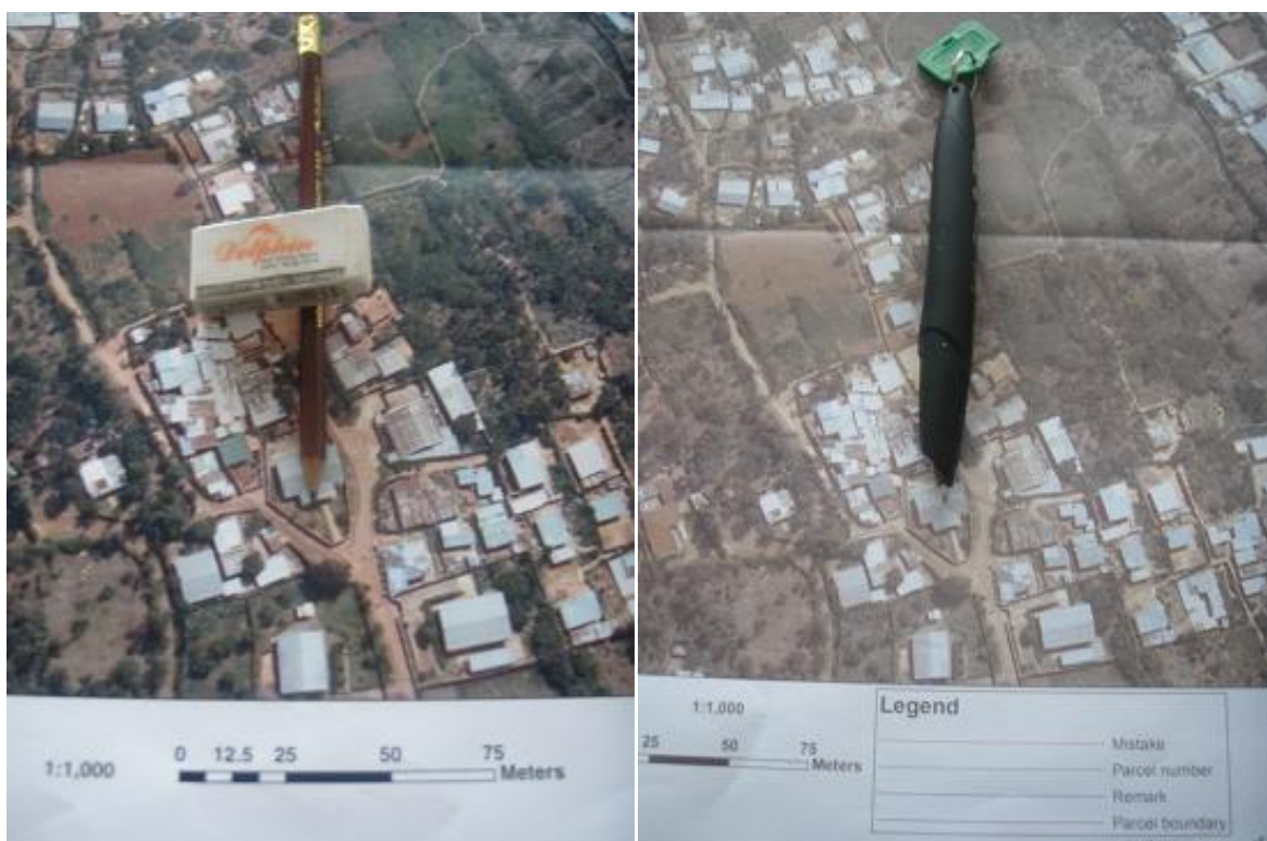
Figure 18. Pencil based (left) and digital pen based (right) for orthophoto based land adjudication
