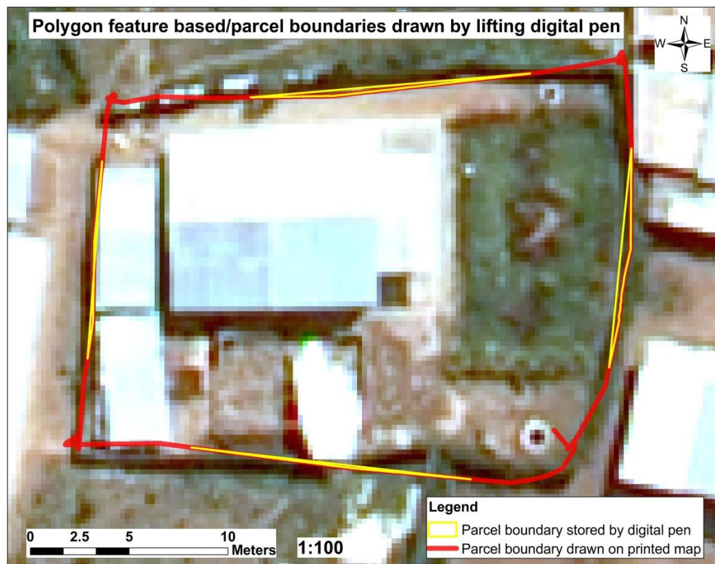
Figure 6. Polygon feature based/parcel boundaries drawn by lifting digital pen
