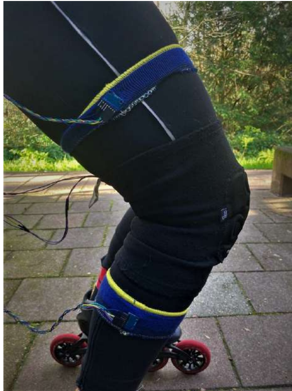
Figure 4.10: The set-up for the durability test. The flex sensors are underneath the knee protection.
