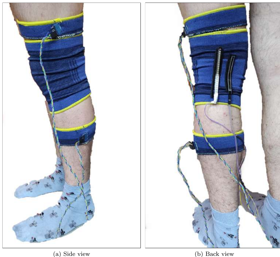
Figure 4.8: The set-up to measure the accuracy of the sensors. The IMUs were positioned on the side of the upper and lower leg. The flex sensors were attached to the back of the knee using velcro and a knee guard.
