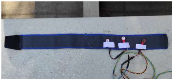
(a) The velcro band with vibration motors on them. With the white short pieces of velcro, the position of the location motors can be adapted.
