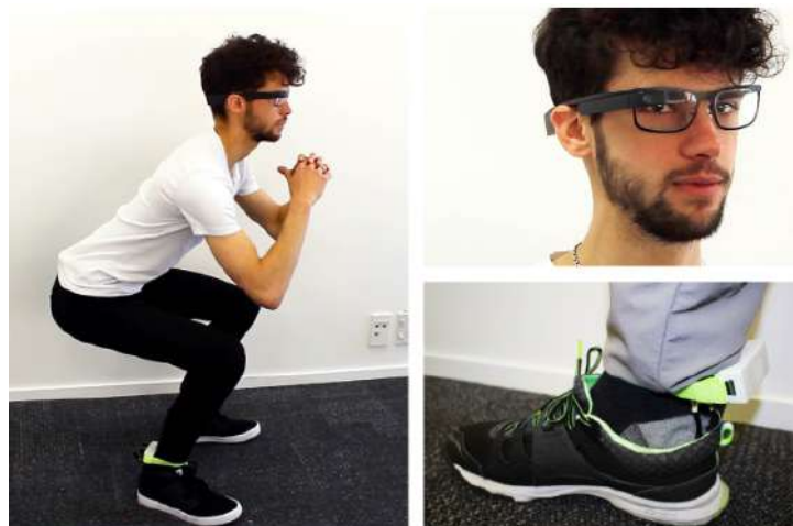
Figure 2.5: The designed GymSoles++. The shoe is incorporated with an insole to calculate the body's centre of pressure (CoP) and 8 vibration motors. The vibration motors provide haptic feedback and the Google Glasses provide visual feedback on the CoP of the user. [20]
