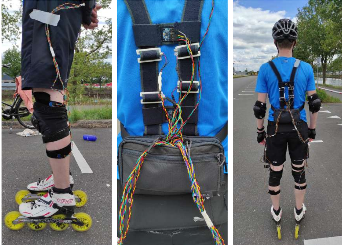
(a) IMUs placed on the right leg. One IMU is placed above the joint and one below. Underneath the knee guard, the vibration motor is placed. (b) IMU placement on the back to measure whether a person has a round back or not. The four white clips are where the vibration motors are positioned. (c) Full setup from the back. On the right shoulder, a motor for a 'pat on the back' is located.
