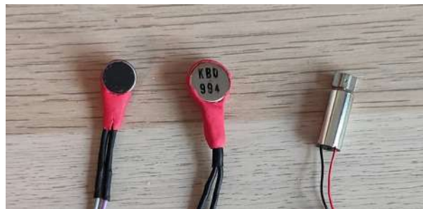
Figure 7.1: The three vibration motors which were used throughout the experiments. The vibration motors are ordered from left to right on vibration strength. The first two coin motors were too weak to perceive during inline skating. The cylindrical motor can be perceived during inline skating.
