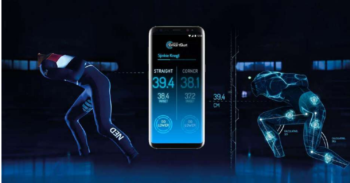
Figure 2.13: Image of the Samsung SmartSuit. The suit contains five sensors which communicate with an app. Via the app, the coach can press on the "Go Lower" button, which sends vibrotactile feedback to the wrist of the athlete.
