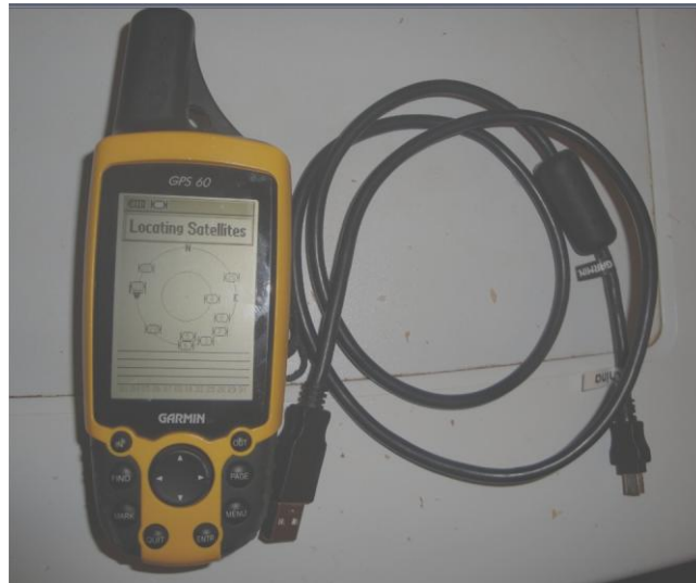
Figure 5-2: Hand held GPS (Garmin GPS 60). Accuracy + or - 7 meter.
