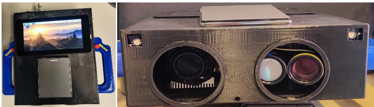
Figure 3 Left: top view of the WIPI. Right: front view of the WIPI with the laser in the left window and the mono camera (left) and colour camera (right) in the right window. Two LEDs are mounted in the upper corners.
