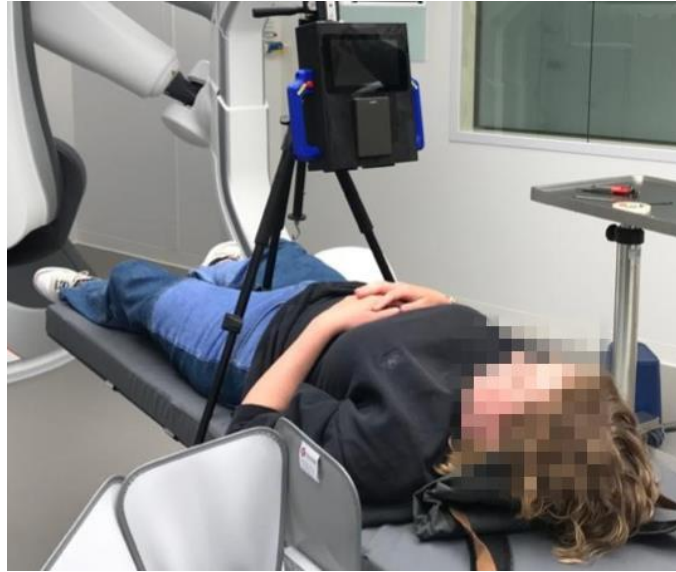
Figure 7 The set-up of the mounted measurement at the middle of the abdomen with the WIFI held in a tripod.
