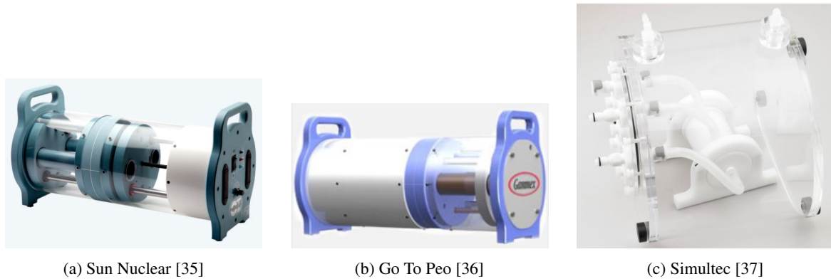
Fig. 3.3 Commercially available perfusion phantoms
