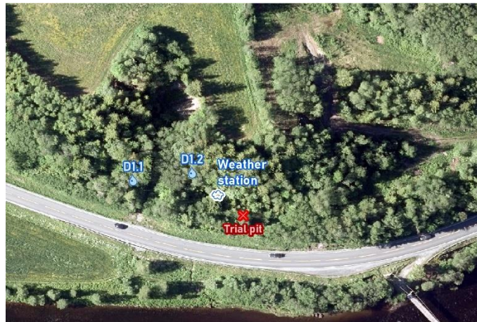
Figure 5. Location of monitoring devices (D1.1 and D1.2) and weather station installed in Kjellberget during the KlimaDigital project (Depina et al., 2021). Also featured in the image is a trial pit site excavated to obtain soil samples. Background image: Stjørdal 2015 – norgebilder.no.
