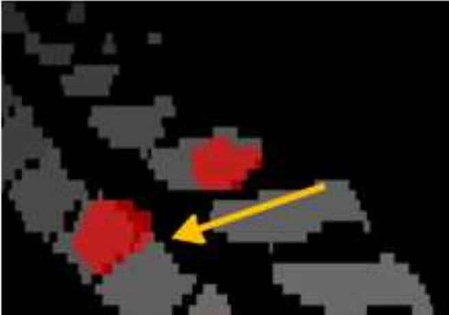
Figure 8: Example of incorrect segmented voxels
