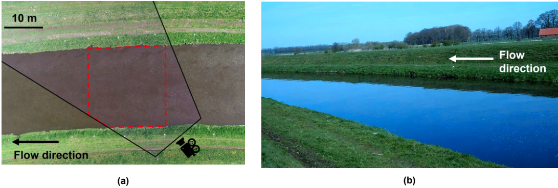
Figure 3.44: Location 3 at the Dinkel River: (a) drone-view of location 3, the solid black box represents the FoV of the stationary camera and the dashed red box delineates the ROI considered for the comparison between drone-based and fixed camera LSPIV; (b) snapshot of the video recorded by the stationary camera.
