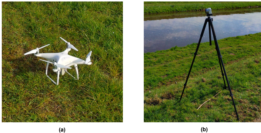
Figure 2.14: Experimental setup Dinkel River: (a) DJI Phantom 4 Pro drone; (b) stationary camera setup.
