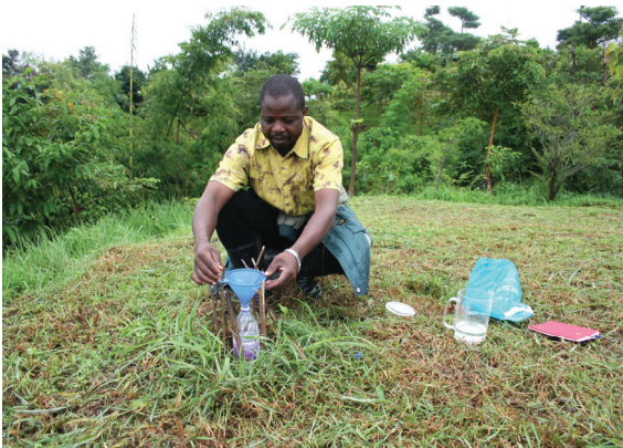
Figure 3-3: Putting up a rain gauge to measure rain at one of the points in the catchment (X: 721266,Y:1856276)
