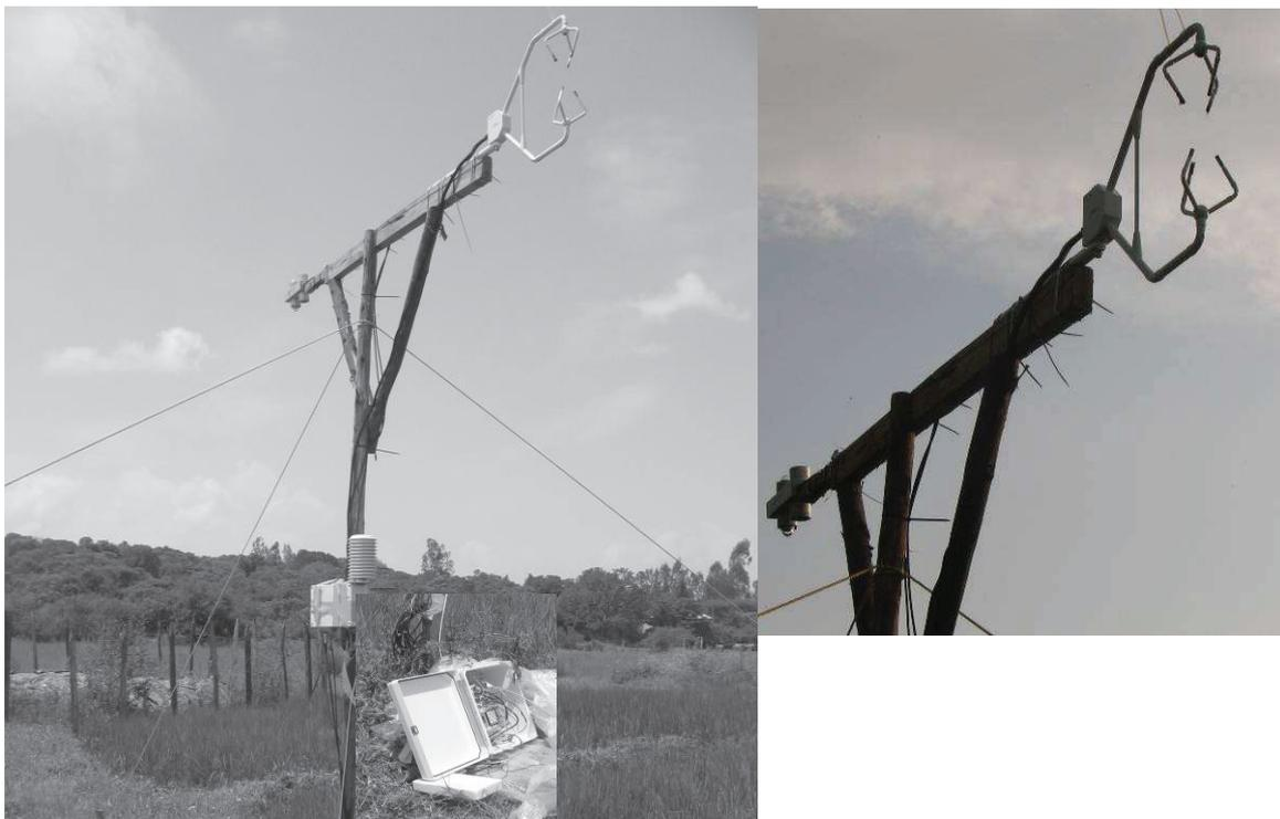
**Figure 3-4** Flux tower installed during the field campaign
