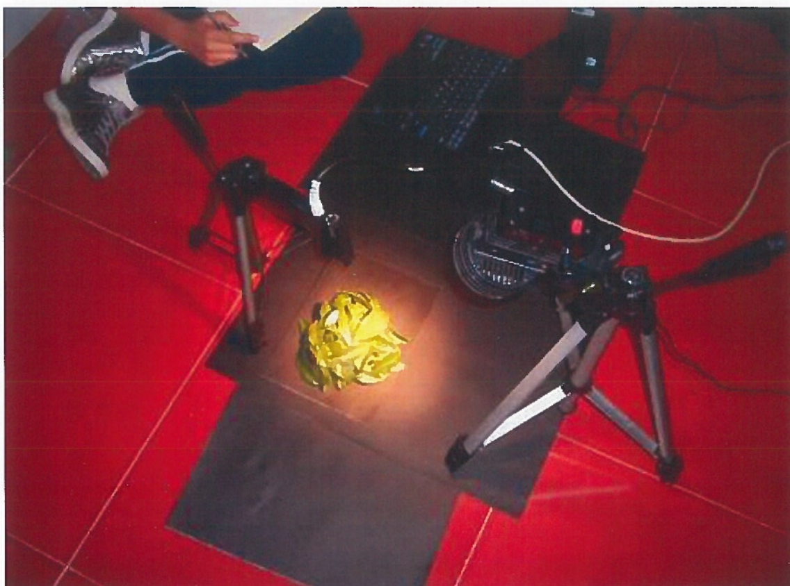
Figure 2.2 Experimental setup for spectral measurements of fresh tea leaves
