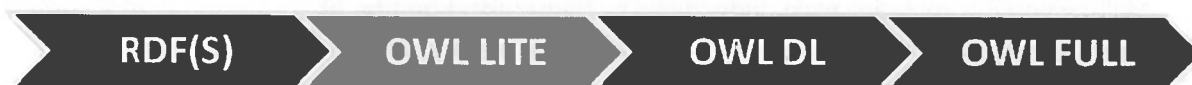
Figure 36. Increasing the amount expressiveness and computational complexity. From left to right, the right one include the left one both semantically and syntactically
