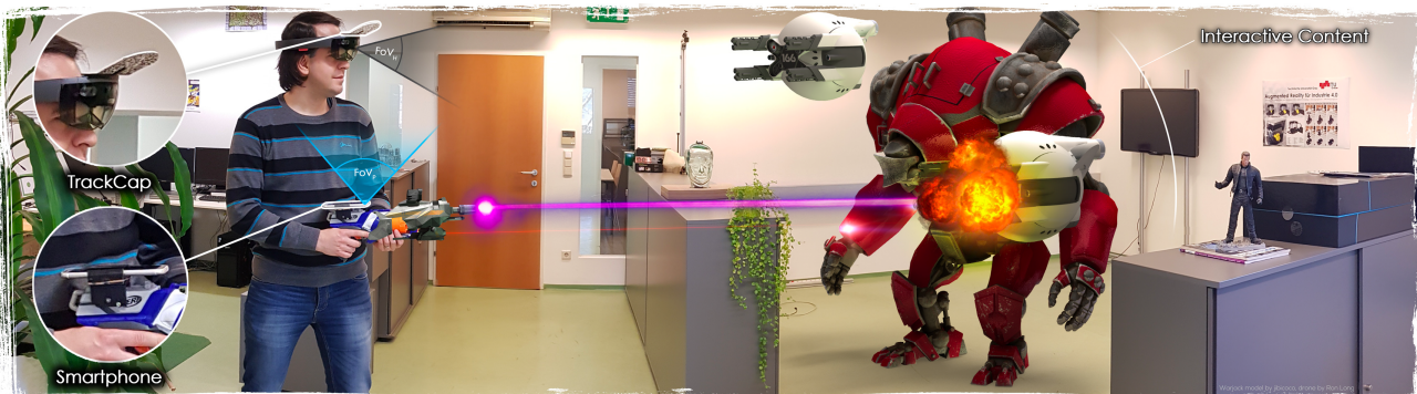
Figure 2.3: TrackCap(2019) uses the smartphone as a precise 6DOF input device for ARHMD
