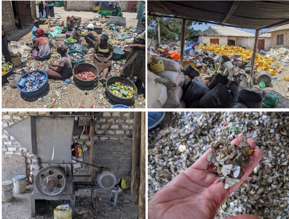
Figure 18. A CBO in Mombasa. In clockwise direction: Women sorting plastic by type and colour; plastic sorted by type and color, waiting to be sold (bought from individual collectors); the machine used to shred plastic, reducing the volume; hard plastic after being crushed.
