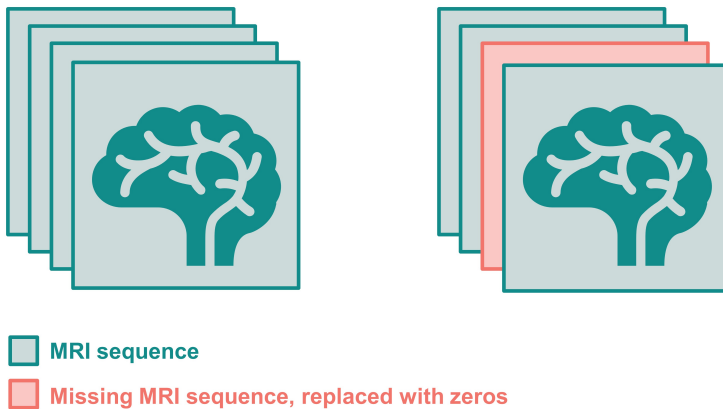
Figure 4.5: Dealing with missing sequences in multisequence data. Missing sequences are replaced by zeros to ensure a uniform scan size.
