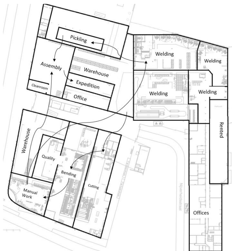
Figure 3: Facility Layout Map company Y (The arrows show the flow of articles through the facility)
