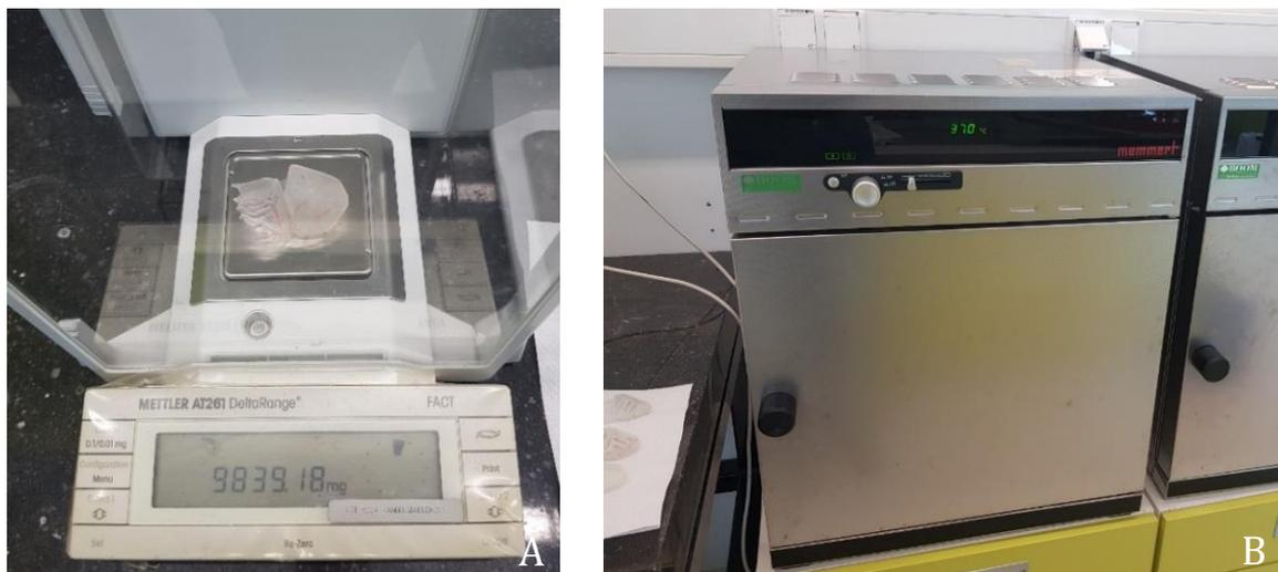
**Figure 4.2.** Experiment tools. **A)** Material weighting using the Mettler-Toledo analytical balance. **B)** Stove with the prosthesis placed in 37° Celsius heated water.
