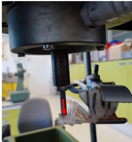
**Figure 4.3.** Vertical applied load (red arrow) on the fixated obturators using the Instron 6022 machine.
