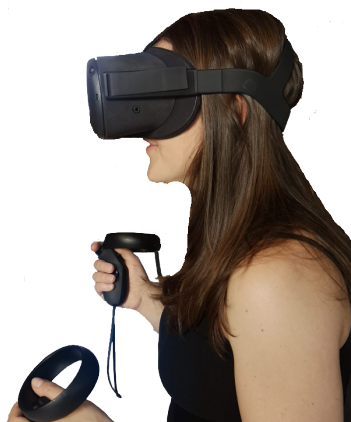
Figure 2.1: Example of a VR head-mounted display with controllers: Oculus Rift [8]
