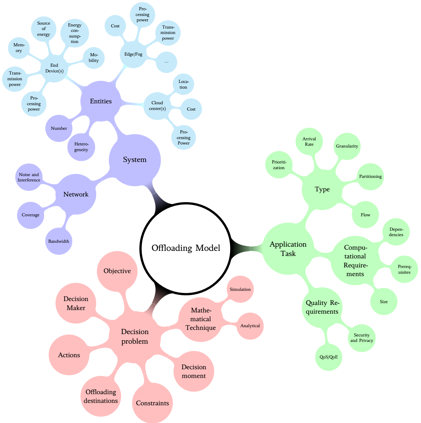
Figure 2.4: Classification of factors involved in modelling the offloading decision problem.
