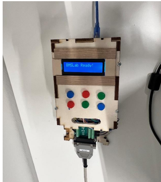
Figure A10. Device used to facilitate the communication between Unity and the Amplifier
