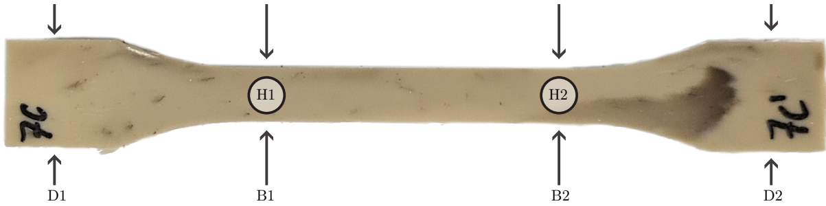
Figure 3.7: Example of a moulded dogbone specimen according to ISO 20753-12A
