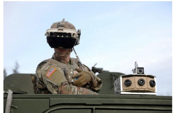
Figure 11. A soldier wearing the IVAS; on the bottom right are cameras that provide vision for passengers through their HMDs
