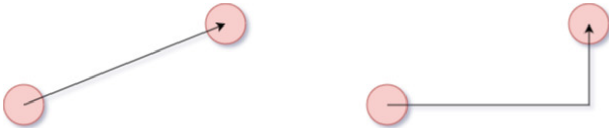
Figure 3-9 Euclidean (left) and rectilinear (right) distance
