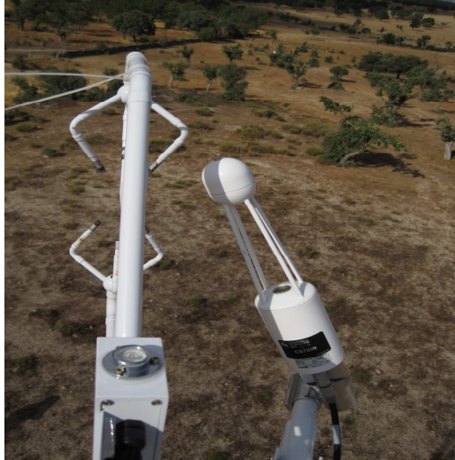
Figure 3-3 : a) To the left side is CSAT-3(Campbell Scientific, 1996) and CO 2 /H 2 O gas analyser LICOR L1 7500, b) to the right side includes all CSAT-3, CNR 1 Net Radiometer (Kipp & Zonen) and Vaisala in eddy tower Sardon, Spain.
