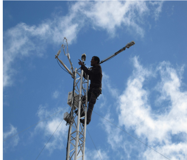
Figure 3-3 : a) To the left side is CSAT-3(Campbell Scientific, 1996) and CO 2 /H 2 O gas analyser LICOR L1 7500, b) to the right side includes all CSAT-3, CNR 1 Net Radiometer (Kipp & Zonen) and Vaisala in eddy tower Sardon, Spain.
