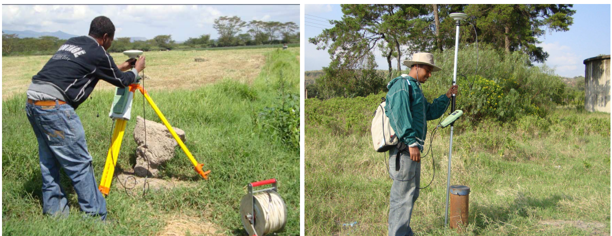
Figure 3:2 Locating the reference station (left) and well top elevation survey (right)
