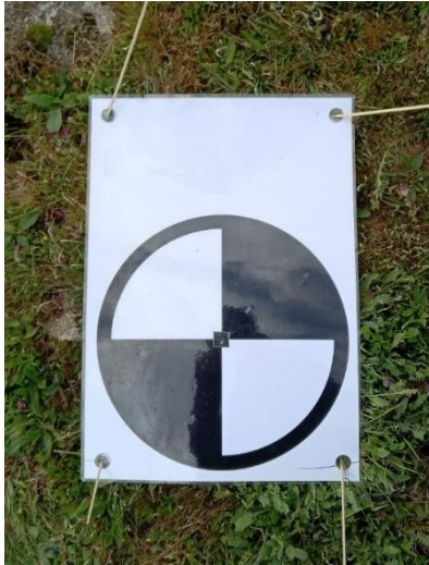
Figure 6: Target mark used as GCP in the study area
