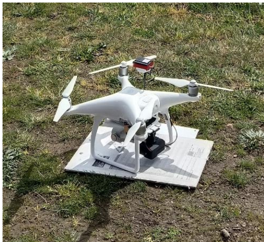
Figure 5: DJI Phantom 4 with sequoia camera and sunshine sensor in the field.
