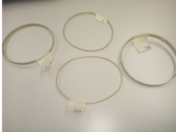
Figure 4.7: Obtained geometries after long continuous printing at different printing. This tests confirms convergence to set point of 0.66 since all geometries have ultimately the same line width.
