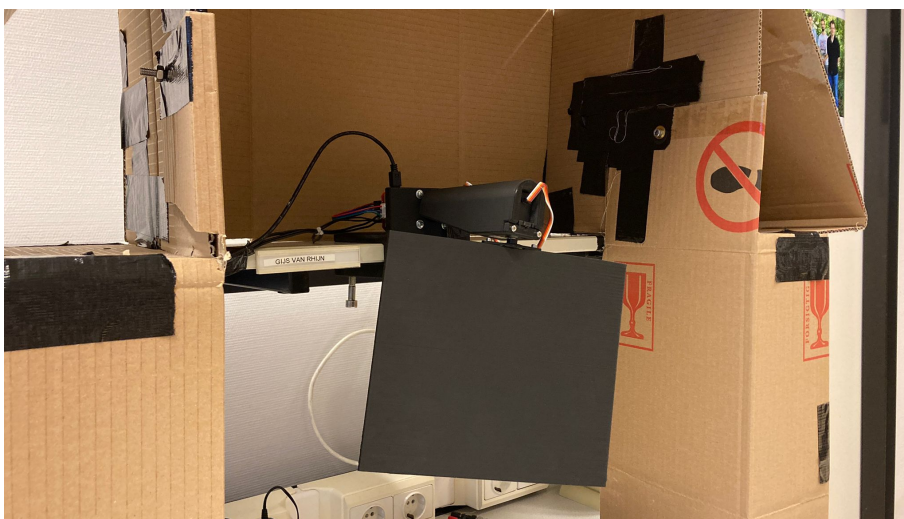
Figure 3.3: Image of the placeholder flapping wing setup surrounded by a protection cardboard cage.
