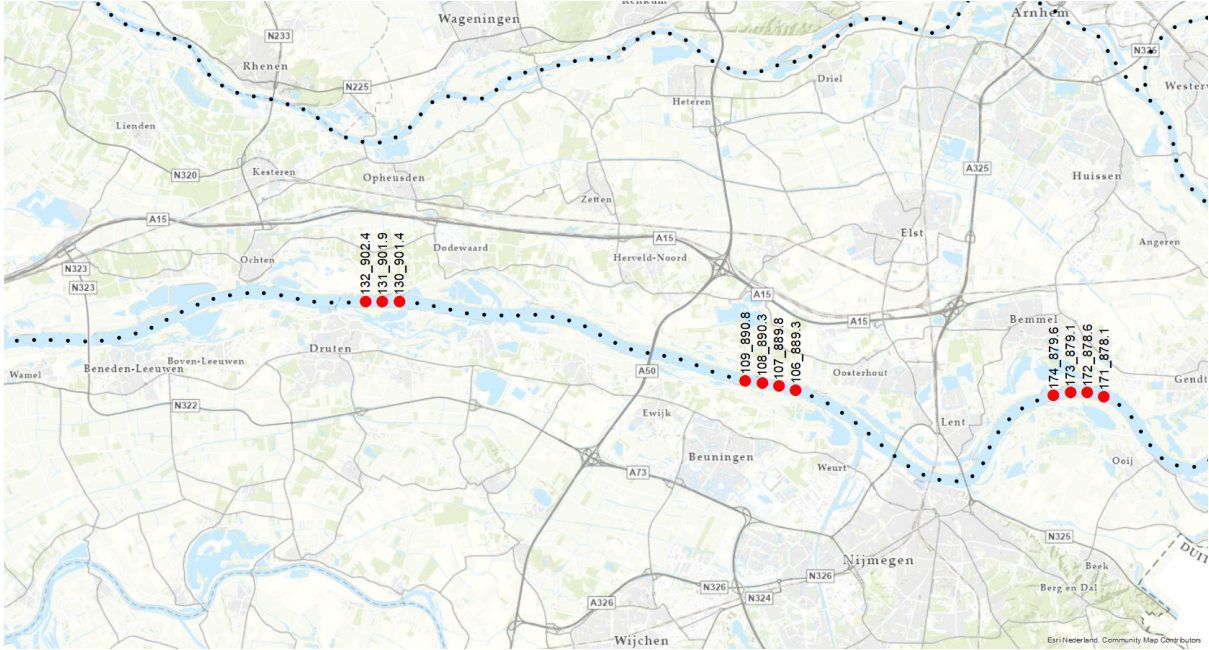
Figure A.13: Simulation 8. Nourishment in the Boven-Waal & Midden-Waal; rkm 878-880, rkm 889-891 & rkm 901-902.5. The label indicates the node ID and the chainage of the node according to the format 'ID_Chainage'.
