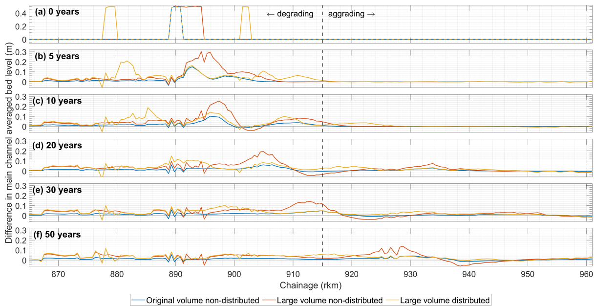
Figure 4.23: Difference in main channel averaged bed level in the Boven-Rijn and Waal for the different nourishment volumes compared to the reference simulation at different moments in time. The approximate location at which the trend changes from degrading to aggrading in the reference simulation is indicated as a dashed line at rkm 915. Mind the difference in scaling between subfigure (a) and subfigures (b-f).
