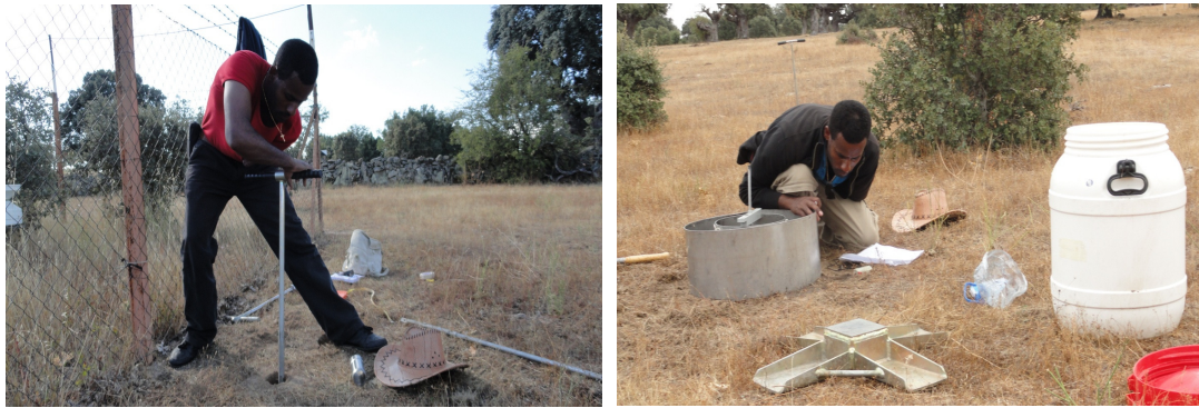
Figure 6. Auguring for soil sampling and study of water table depth (left) and infiltration test to estimate in situ vertical saturated hydraulic conductivity of the soil (right)
