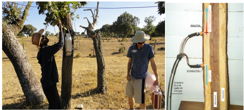
Figure 9. Installation of sap flow measurement (left) and arrangement of TDP in a tree (right), source (Mapanda 2003)
