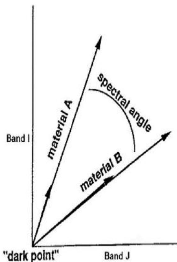
Figure 3. : Two-dimensional illustration on the concept of SAM algorithm (Margate and Shrestha, 2001)
