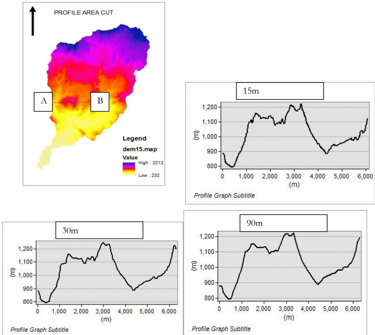
**Figure 16. Profile cut and profile graphs of DEMs from average aggregation**
