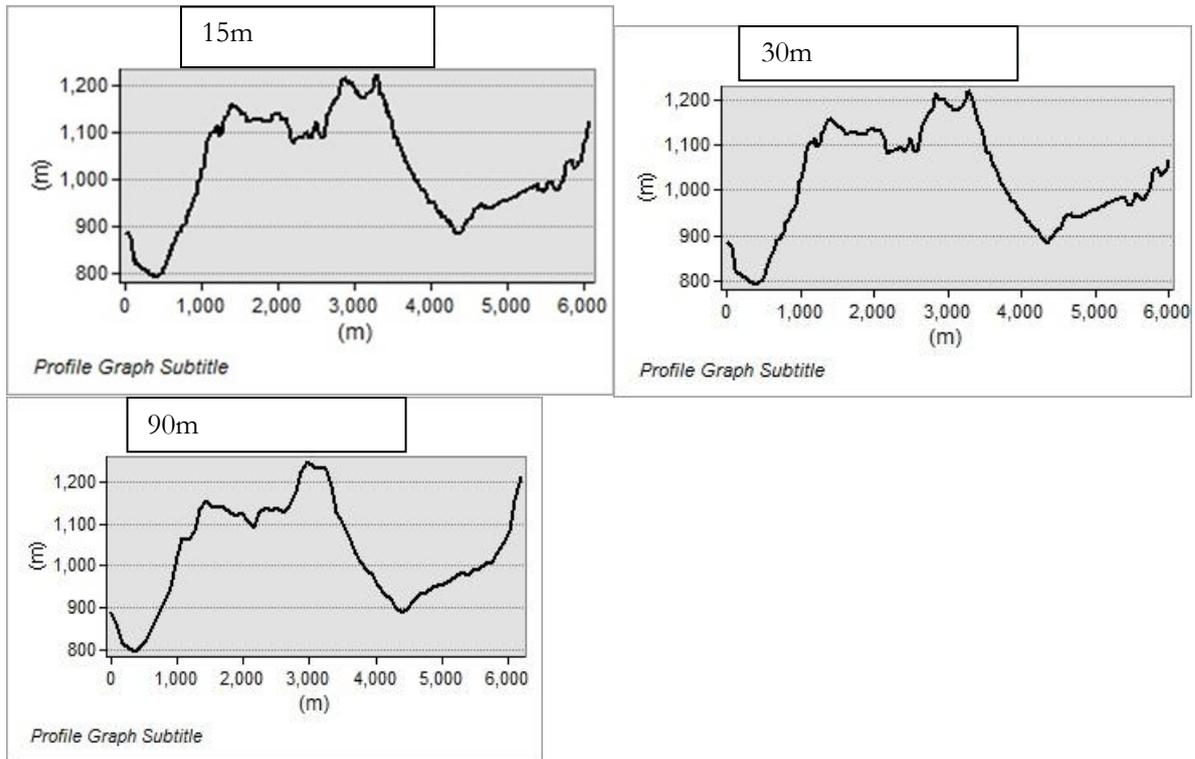
**Figure 18. Profile graphs of DEMs from median aggregation**
