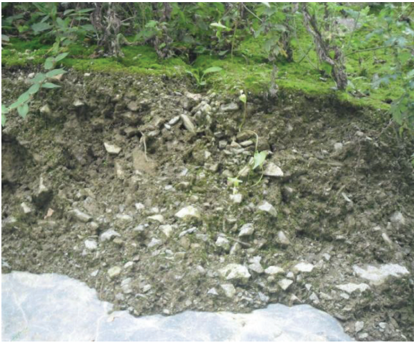
Figure30 show where soil sampling failed due to stony nature of the soil
