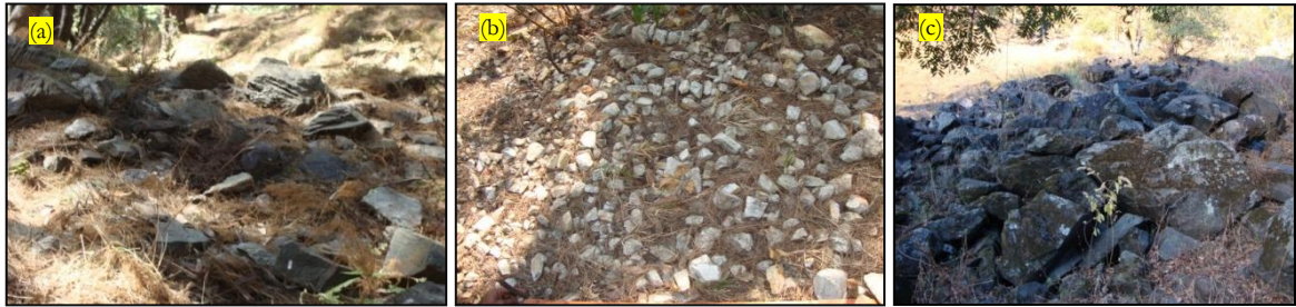
Figure 4-11: Surface roughness measured at rockfall sites-(a) Gagnani, (b) Hinna and (c) Aungi
