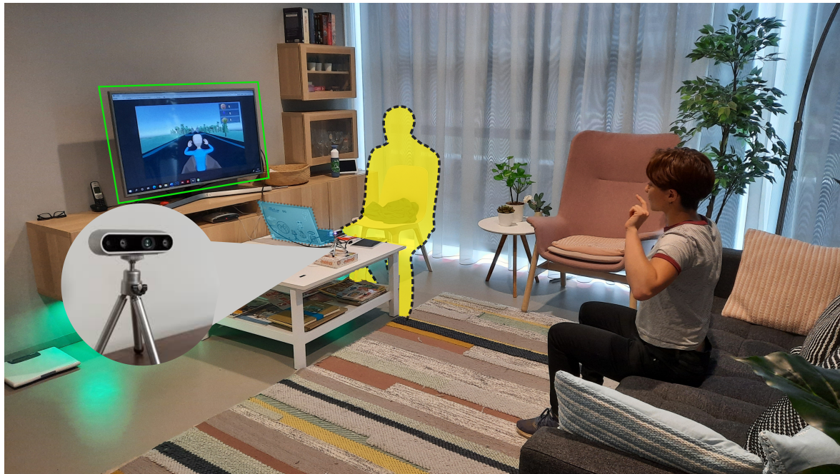
Figure 6.1: Experiment set-up. (Blue)The laptop with the developed exergame was connected to the television in the living room. (Pop-out)The depth camera d435i was placed at a height of 70 cm from the ground and 2 meters from the couch. The height of the couch was 53 centimeters from the ground. (Yellow)The researcher was sitting next to the laptop, observing both the game and the participant
