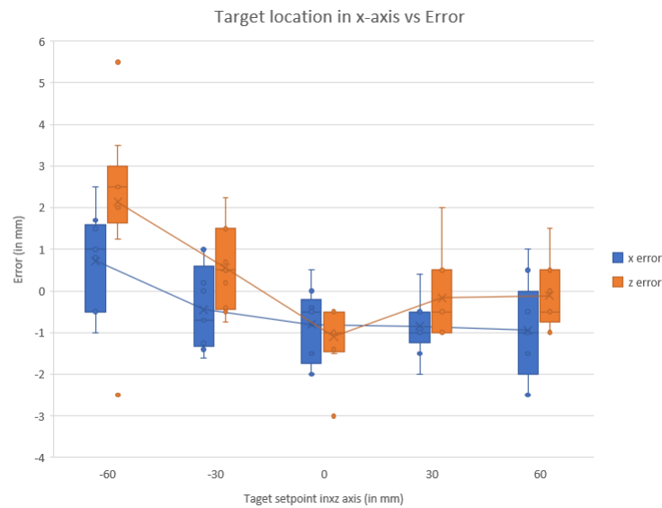
Figure 5.10: Targeting error along x and z versus target coordinate displacement in x axis
