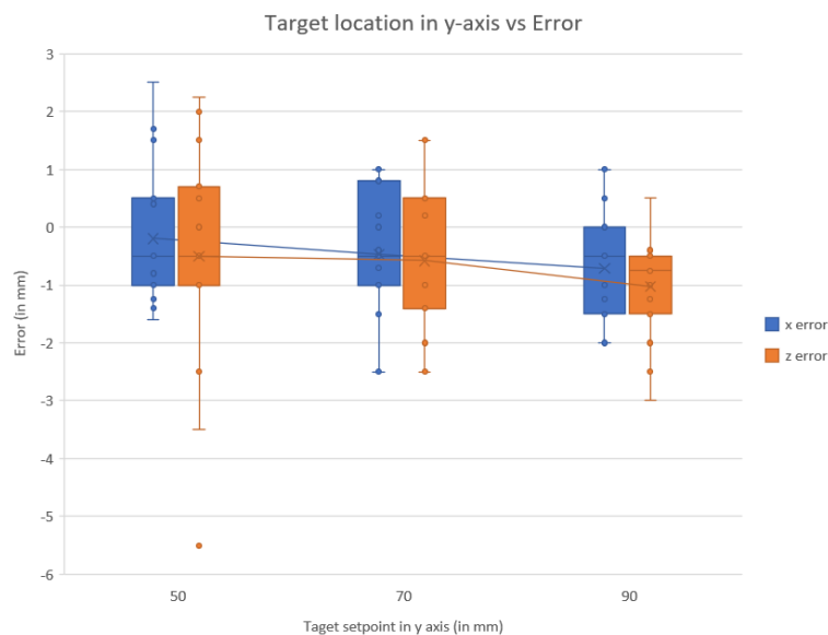
Figure 5.11: Targeting error along x and z versus target coordinate displacement in y axis
