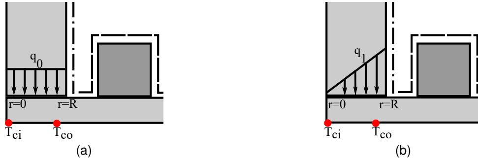
Figure 4.3: Schematic of the heat flux distribution with thermocouple inside ( T_{ci} ) at (-4, 0) mm and thermocouple outside ( T_{co} ) at (-4, 8) mm: (a) zero order, (b) first order
