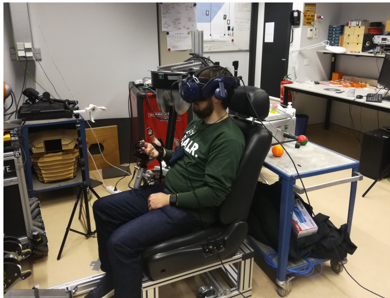
Figure 3.1: Telerobotic setup on the master side, including a Virtuose 6D and HGlove.
