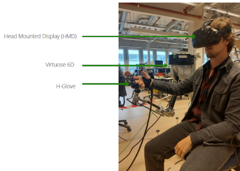
Figure 1: Operator wearing haptic devices and HMD.
