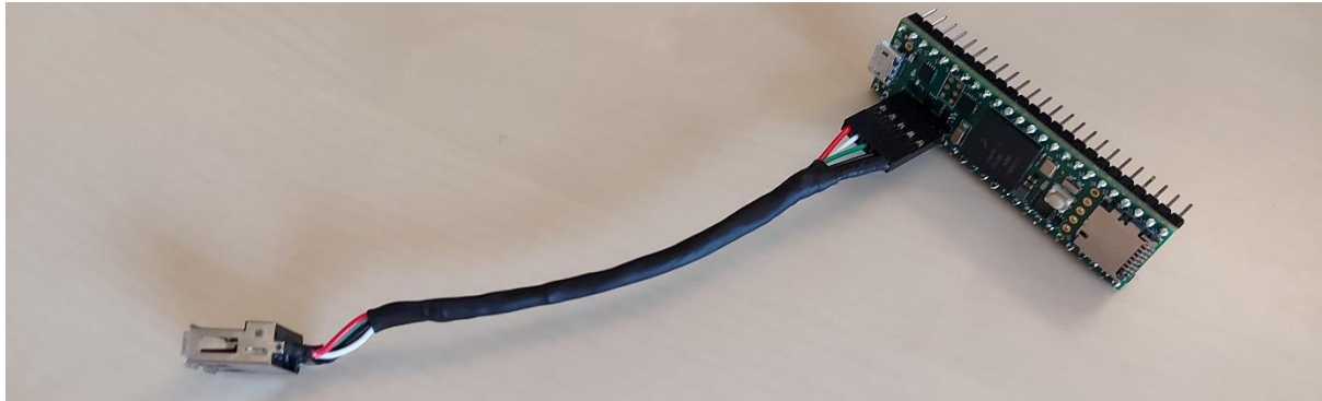
Figure 23, the full image of connecting a USB A female header to T3.5
