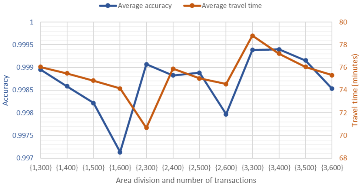
Figure 4.16 Performance of parameter values for location- and opportunity-based cycle counting in the bulk storage
