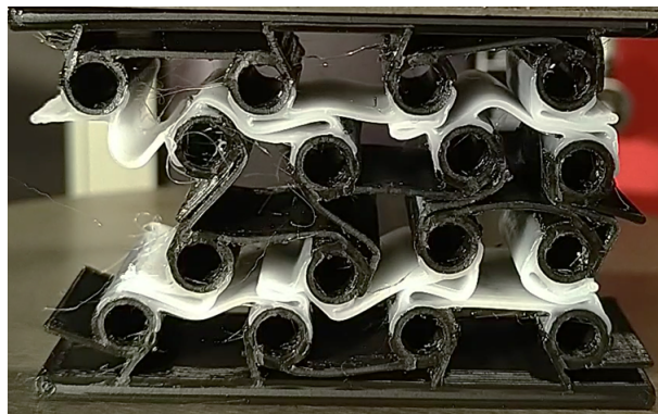
Figure 4.16: Different deformation behaviour of one out of three SHS structures.
