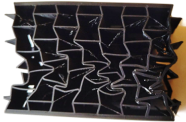
(g) Failure mode re-entrant from strain rate experiment in section 3.5
