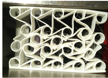
(e) buckling behavior of chiralN6
