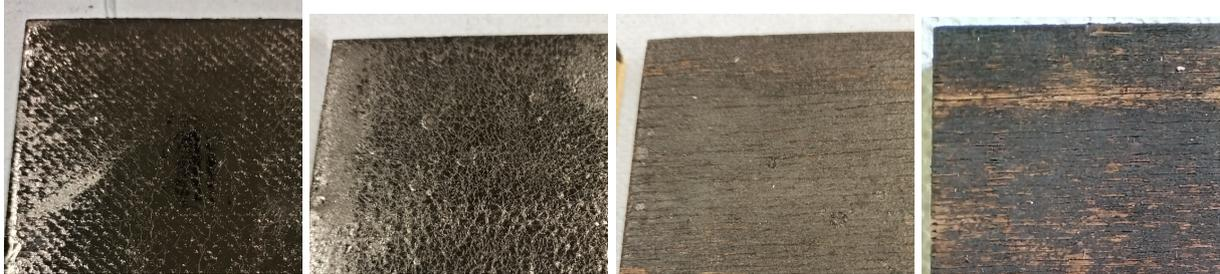
Figure 11: Cropped images of the WTP coated samples to visually compare natural weathering effects. Left to right: 0 (reference), 7, 28, and 77 days natural weathering.
