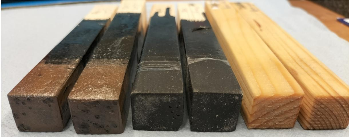
Figure 29: Picture of the submersed samples taken after 14 days. Left to right: woody theroplastic, ‘Rambo’, and bare wood.
