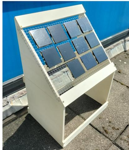
Figure 3: Picture of the natural weathering setup. The samples are stapled to the chicken wire at the back. The rack is angled  $45^\circ$  and faces south.
