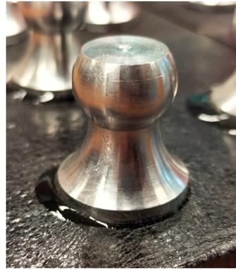
Figure 5: Image of the dolly glued to the coating.
